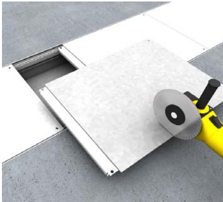
34 | Dummy cover section Cut the cover part (L < 500 mm) to the required length.
