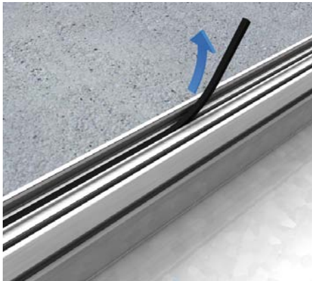
37 | Duct system for wet-cleaned linoleum floors Remove the rubber insert (UEBSPGD) from the side profile of the duct completely.
